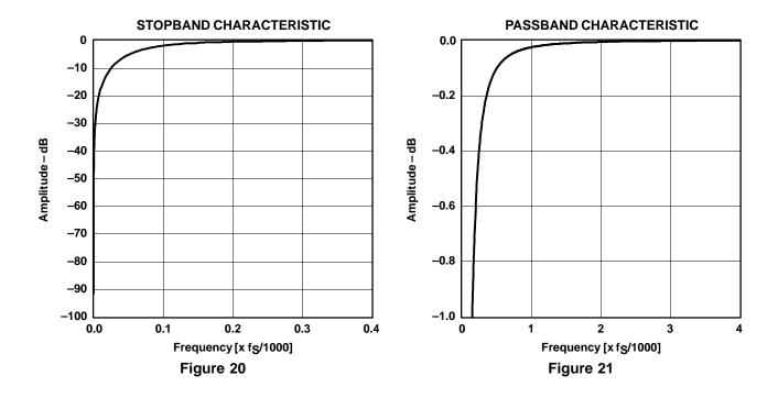
ADC ANALOG ANTIALIASING FILTER FREQUENCY RESPONSE
